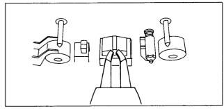
After much use, slight magnetism can build up on the recording and playback head causing loss in high frequency sound and increases in noise. To eliminate this problem you should periodically demagnetize the head with the optional accessory Head Demagnetizer AH-15. Damagnetize the metal parts of the capstan as well.
